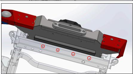
Then simply hold the Splash Guard up under the bottom of the Modular Front Bumper, and install the hardware using (8) M4x16mm Button Head Flange Bolts.
